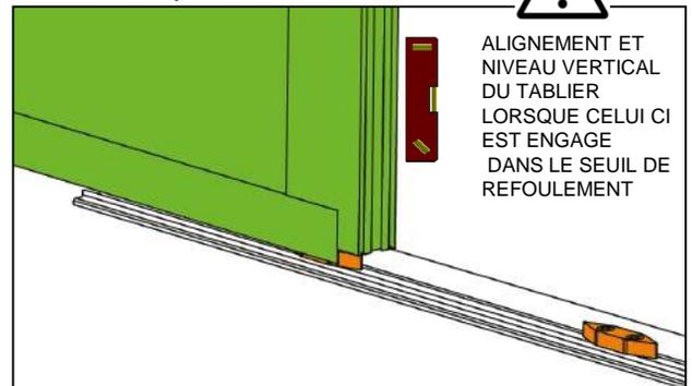
ALIGNEMENT ET NIVEAU VERTICAL DU TABLIER LORSQUE CELUI CI EST ENGAGE DANS LE SEUIL DE REFOULEMENT
